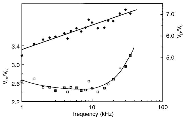
**Fig 2.** The variation in relative threshold with MFAC frequency. MFAC 10-ms bursts applied at a burst frequency of 50Hz with small electrodes ( $3.2\text{cm}^2$ ). Legend:  $\square$ , motor threshold/sensory threshold ( $V_m/V_s$ );  $\blacklozenge$ , pain threshold/sensory threshold ( $V_p/V_s$ ).
