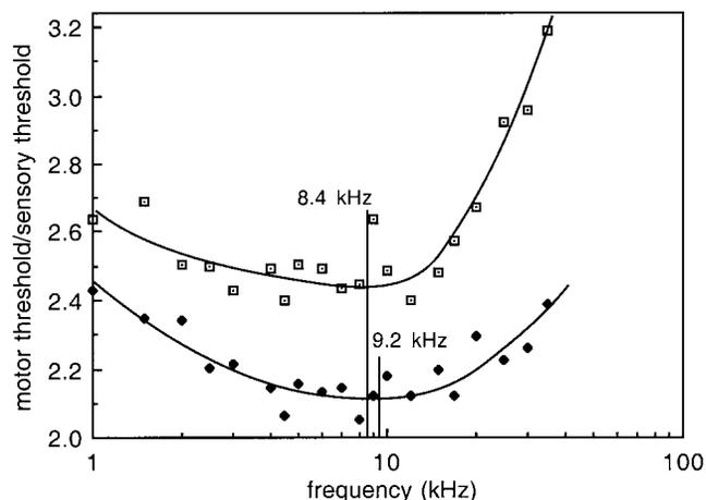
**Fig 4.** The variation in motor threshold/sensory threshold ( $V_m/V_s$ ) with MFAC frequency. Minimum relative threshold frequencies are shown for each. Legend:  $\square$ , relative thresholds using small electrodes and 10-ms bursts of MFAC at 50Hz;  $\blacklozenge$ , relative thresholds using large electrodes and single-sinewave stimuli at 50Hz (present study).
