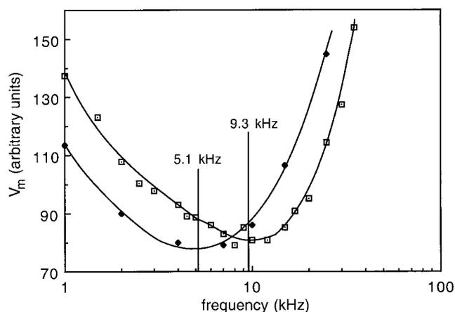
**Fig 1.** The effect of electrode size on the variation in motor threshold ( $V_m$ ) with MFAC frequency. MFAC 10-ms bursts applied at a burst frequency of 50Hz. Minimum threshold frequencies are shown for each. Legend:  $\square$ , small electrodes ( $3.2\text{cm}^2$ );  $\blacklozenge$ , large electrodes ( $17.6\text{cm}^2$ ).
