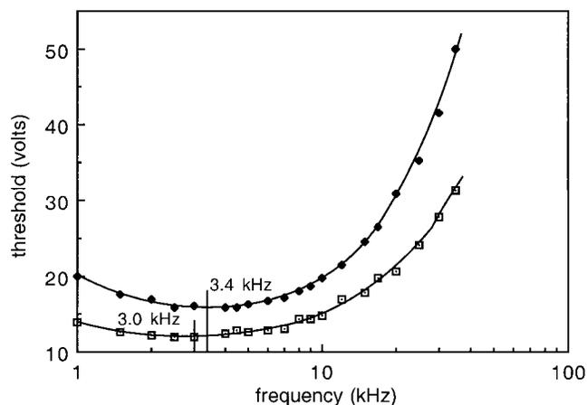
**Fig 3.** The variation in sensory and motor thresholds with MFAC frequency. Single-sinewave stimuli applied at a frequency of 50Hz using large electrodes ( $17.6\text{cm}^2$ ). Minimum threshold frequencies are shown for each. Legend:  $\square$ , sensory threshold ( $V_s$ );  $\blacklozenge$ , motor threshold ( $V_m$ ).
